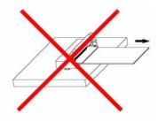
Do not add the load mating FPC/FFC with connector housing.
